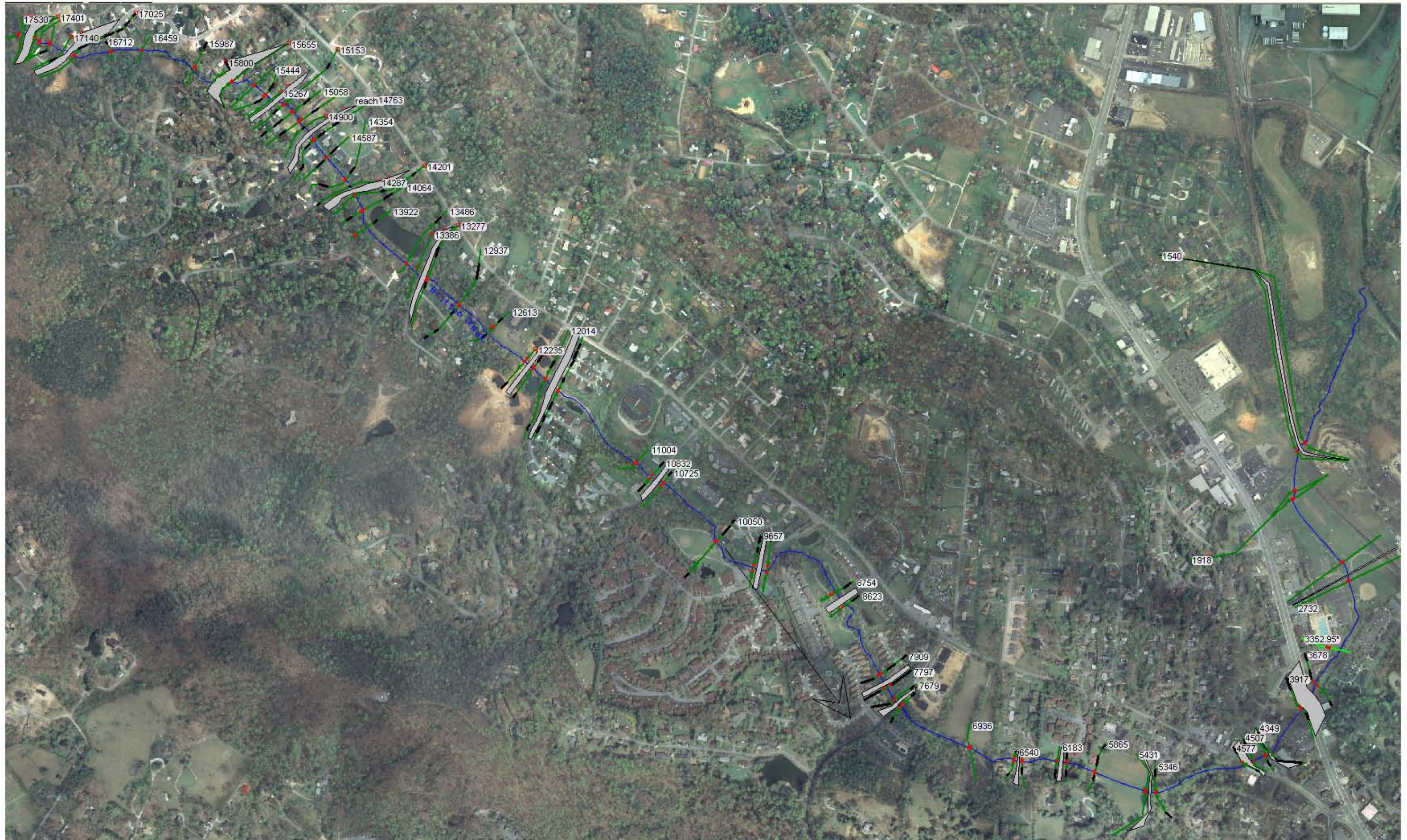
FIGURE 4.4: SCREEN SHOT OF HEC-RAS GEOMETRY FOR BRITTON CREEK. NUMBERED CROSS SECTIONS ARE GREEN. ROAD CROSSINGS ARE GREY. BANK STATIONS ARE RED. STRUCTURES IN CROSS SECTIONS ARE BLACK.
